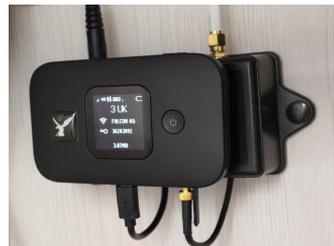
Turn on the power on the 4G docking station, the light on the switch should illuminate to confirm power on.
