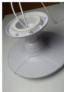
When positioning the antenna to on the roof, firstly pass the DTV cable through the roof followed by the 4G cable. Add the adhesive to the base of the antenna and position the antenna and align with the previously drilled holes ready for securing to the antenna to the roof.
