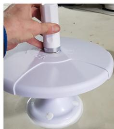
Screw the 4G module to the top of the Antenna.
