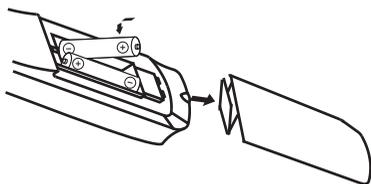
⇒ Insert two batteries into the battery compartment paying attention to the indicated polarities and push the cover of the battery compartment carefully until the cover is locked.
