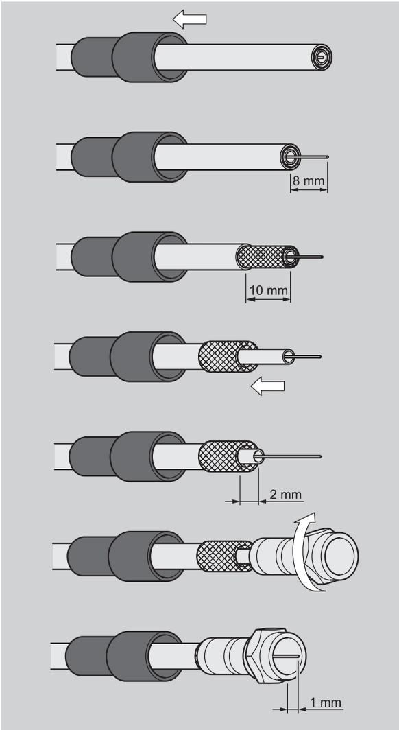
⇒ Fasten the F connector of the coaxial cable onto the “LNB IN” antenna connection of the receiver. Fasten the other end of the coaxial cable to the LNB.
