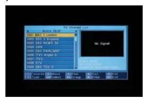
20. Now again check the signal quality and intensity by pressing "info", if over 80% intensity and 65% quality, press "info" to view. If you have high intensity but not so high quality there is most likely an obstruction between the dish and the satellite, i.e. trees
