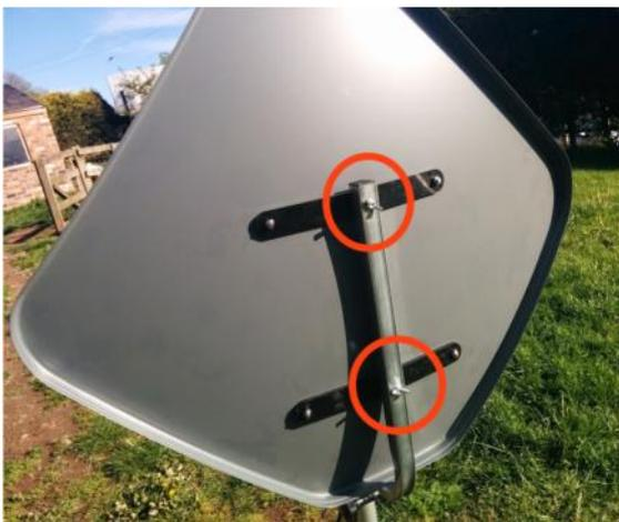
5) Mount the dish on the tripod and use the compass to align one of the tripod legs so that it is in the azimuth direction indicated by the dish pointing table included with the kit.
