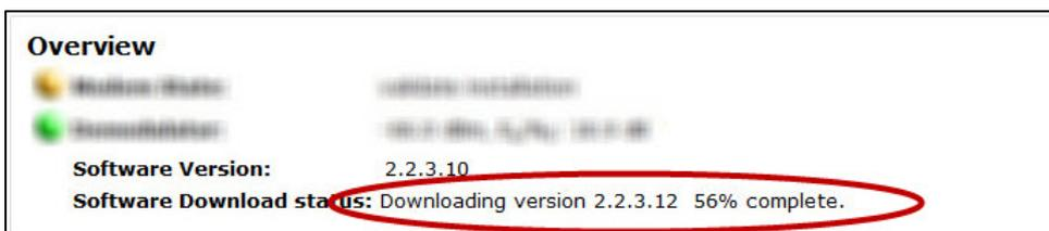
Once the download is complete, the new software is written to flash memory and the modem reboots to activate the new software. You can now proceed to the next step: Validating the Installation.
