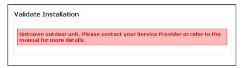
The outdoor unit which was selected on the modem has an ID which is unknown by the hub. Possible reasons:
