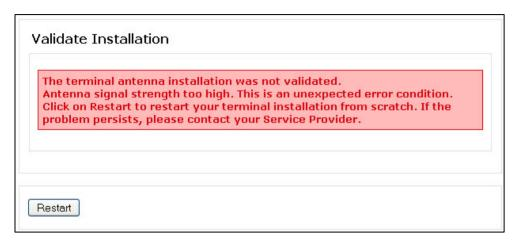
The entered address determines the position of the terminal in the beam and its corresponding maximum signal strength. The measured signal strength is above the maximum acceptable value. This is an unexpected error condition. It can occur e.g. when using an antenna with bigger diameter than the selected outdoor unit type, or when there is a mismatch between the selected outdoor unit on the modem and its corresponding settings in the hub.
