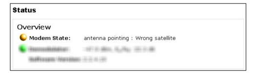
The antenna is not pointed correctly.
