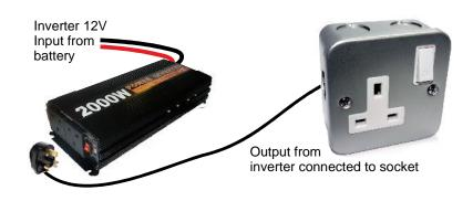
Replace input to consumer unit with 3 Pin mains plug
