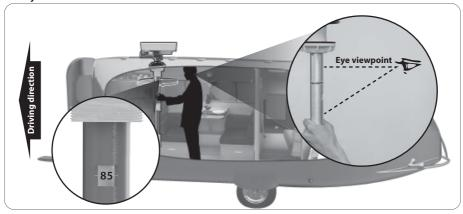
Return the antenna to home position. Elevation indicator has to be faced to the center of vehicle rear to confirm that the azimuth is adjusted to right direction. (HOME position)
