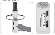
Turn the skew control knob according to the target satellite skew angle.
