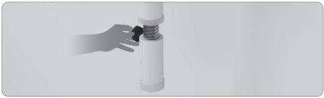
Screw 'Knob Bolt' like the picture below And make skew control knob fixed.
