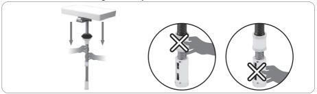
Down the antenna to the ground fully with pole (Do not pull down the antenna by holding elevation screw cap and skew screw cap)
