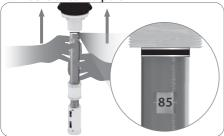
Lift up the antenna pole up to red line to secure enough adjustable space on the roof.
