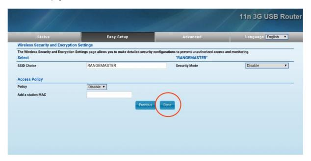
**8.** Wait for the router to reboot, you may need to manually reconnect to the RangeMaster Wi-Fi once it has rebooted and enter 192.168.2.1 in the address bar again.
