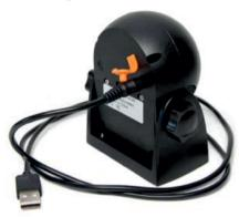
Connect the other end of the charge lead to the included USB to car cigarette lighter/accessory socket adapter or a USB mobile phone adapter.
