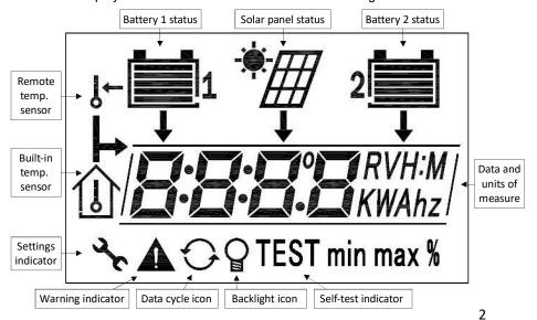
LCD display of the remote meter can show the following information:
