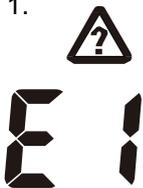
Meaning: Battery polarity reverse warning
