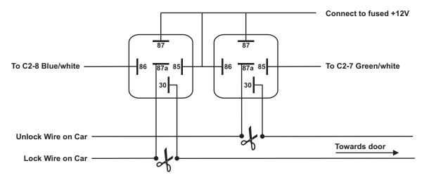
Make sure terminal 30 is connected to the side of the cut wire that goes towards the door motor.
