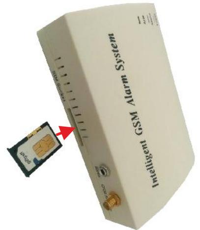
Screw the antenna to the socket on the top of the alarm.
