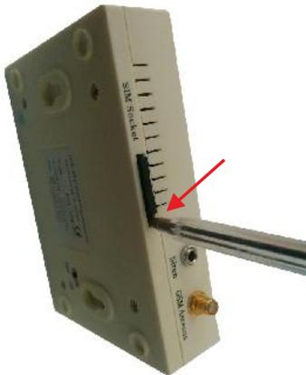
Using the tip of a pen eject the sim card tray from the top of the alarm.
